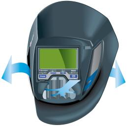
Exhaled air is directed through the four aerodynamic vents. It then exhausts through two thin openings created between the double-shell construction of the heat-reflecting silver front panel and the black helmet.
